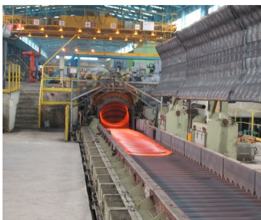
Fig.1. The Stelmor conveyor in the Rod Mill of CSC.
